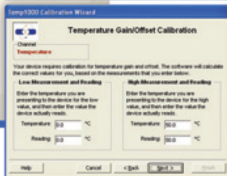
Figure 9: Software calibration adjustment to a logger
