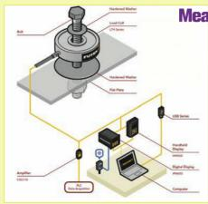
Measuring tightening force with Thru-Hole load cells
